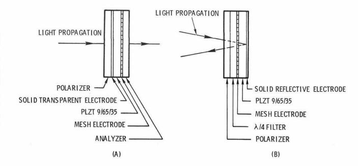
DEVICE CONFIGURATIONS: (A) TRANSMISSION MODE DEVICE; (B) REFLECTIVE MODE DEVICE
